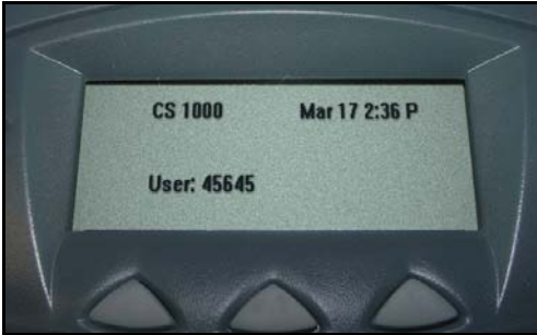
Figure 8: Logged on to an IP Audio Conference Phone 2033 using an IP Phone 2001
