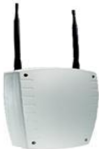
Outdoor Access Point RFP 34
