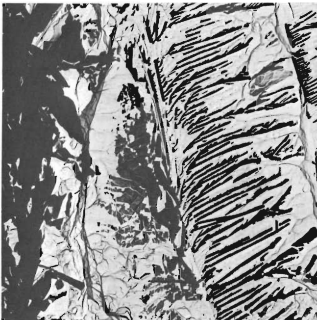
Fig. 9—Electron-extraction fractograph of a CVN impact-test specimen of the ingot of Steel D. Magnification 5700 times.
